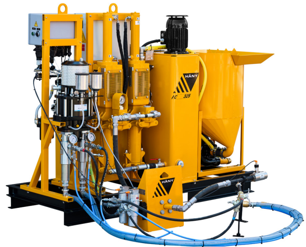
Image 5 CCP plant (combined cement-PU)
