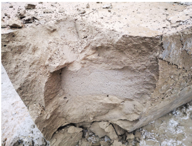
Image 4: Finished cement–polyurethane mixture with RASCOhybrid HMS317
