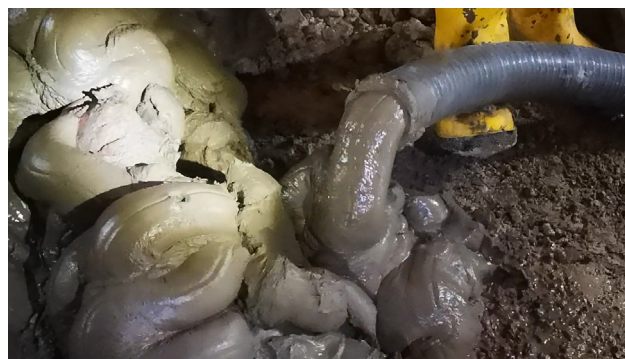
Image 3: 30 m hose test with RASCOhybrid HMS317
